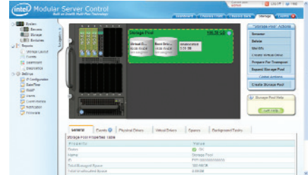
Under the Storage Configuration window, you can create storage pools and virtual drives, as well as map virtual drives to multiple servers using the Intel® Shared LUN feature
